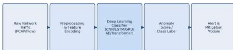
Figure 1. End-to-end deep learning based intrusion detection pipeline
